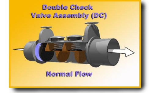
The Double Check Valve Assembly consists of two internally loaded, independently operating check valves together with tightly closing resilient seated shut-off valves upstream and downstream of the check valves. Additionally, there are resilient seated testcocks for testing of the assembly. The DC may be used to protect against a pollutant only. However, this assembly is suitable for protection against either backsiphonage or backpressure.
