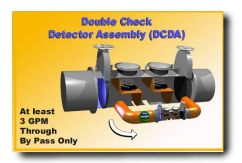
The DCDA is composed of a line-sized double check valve assembly with a specific bypass meter and meter-sized double check valve assembly. The meter registers accurately for very low flow rates to detect any unauthorized use of water. This assembly is used when the protection of a double check valve assembly is required, yet where the added requirement of detecting any leakage or unauthorized use of water exists. Normally these assemblies are reserved for use on fire sprinkler lines.
